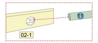
The protruding end of the part 11 needs to correspond to the hole of Section 02-1 when installed. Attach all screws for side 02-1 first and then attach side 02-2
