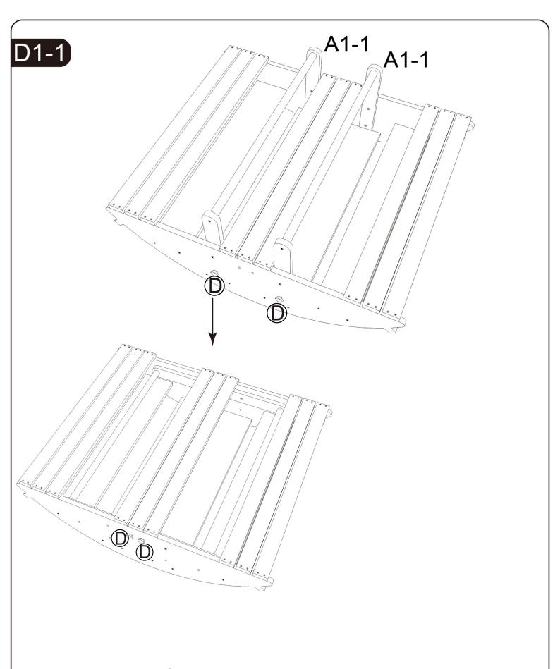
Note: Screw Dout first, turn A1-1 as shown, and tighten screw D
